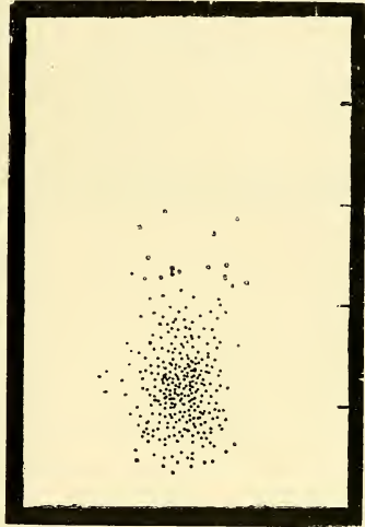
Facsimiles of patterns showing both lateral deviation and stringing of the same pellets.
